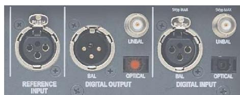
Three I/O formats: XLR, BNC, and optical (Toslink®). All are completely separate from the analog audio XLR connectors, permitting both digital and analog generators to operate simultaneously. No cable changes required to go from A/D to D/A to D/D to A/A testing of a digital tape machine, for example.
