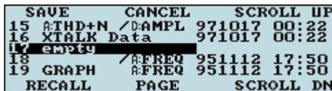
data to be printed or analyzed later. Each saved test includes all settings for the entire instrument, a default description or your own title for the test, the date and time, and the last test sweep result data.
