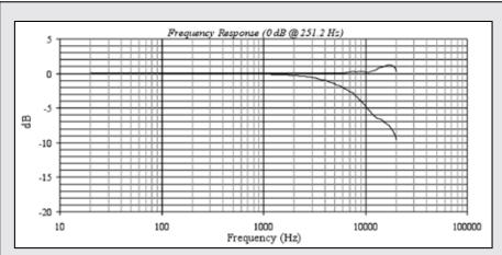
Typical free-field response of the microphone with the grid cap at 0 degree incidence. The top curve is the corrected free-field curve, and the bottom curve is the pressure response generated by the electronic actuator.
