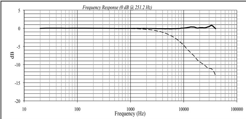
Typical free-field response of the microphone with the grid cap at 0 degree incidence. The top curve is the corrected free-field curve, and the bottom curve is the pressure response generated by the electronic actuator.
