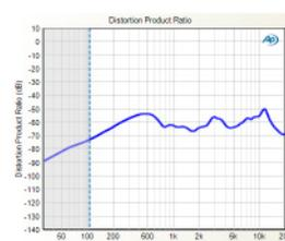
▶ **Distortion Product Ratio:** A display of selected harmonic distortion products as a ratio plotted against frequency. Being able to choose any harmonic from 2<sup>nd</sup> through 20<sup>th</sup> enables more detailed analysis of distortion issues.
