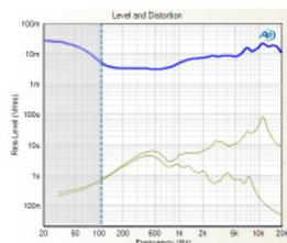
▶ **Level and Distortion:** Both the level vs. frequency and the distortion vs. frequency of the speaker. It's especially useful to have separate traces for the second and third harmonics.
