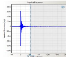
▶ **Impulse Response:** Useful for studying artifacts that move or spread the stimulus in the time domain, such as delay, reverberation, echo, or reflection. An easily adjustable time window is a plus.
