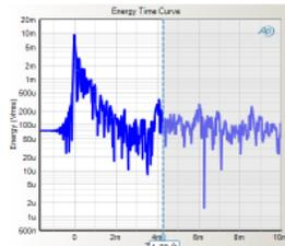
▶ **Energy Time Curve:** The system's energy dispersal in time. Useful for viewing the signal alignment, and for inspecting the arrival of the direct signal, early reflections, and spurious outputs caused by leaks or resonances in the speaker enclosure.
