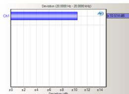
▶ **Deviation:** The total range of level variation across the frequency range. Controls to specify a minimum and maximum frequency range to consider in the deviation measurement are useful.
