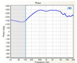
▶ **Phase:** A graphical display of phase vs. frequency. Important for tracking down driver, cabinet, and cross-over problems.
