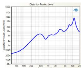
▶ **Distortion Product Level:** A display of selected harmonic distortion products as a level plotted against frequency. Being able to choose any harmonic from 2<sup>nd</sup> through 20<sup>th</sup> enables more detailed analysis of distortion issues.
