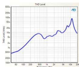
▶ **THD Level:** The total harmonic distortion of a speaker plotted against frequency.
