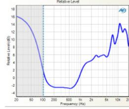
▶ **Level - Relative (frequency response):** Like level, except that instead of absolute units, it is measured in relative units with the 0 dB point determined by the user.
