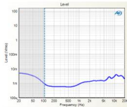
▶ **Level - Absolute (frequency response):** Features such as averaging and smoothing help to remove insignificant response variations that make the general trend hard to see. A shaded area that indicates indeterminate data due to the length of the time gate is valuable.
