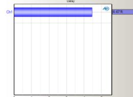
▶ **Delay:** The acoustic delay as sound travels from the speaker to the measurement microphone. This is primarily useful for setting up an acoustic response test.
