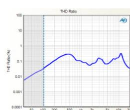
▶ **THD Ratio:** The ratio of the total harmonic distortion to the total signal, plotted against frequency.
