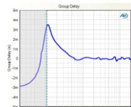
▶ **Group Delay:** A measure of the rate of change of phase shift as a function of frequency. Group delay can also be described as a time delay of a group of frequencies with respect to the generator.
