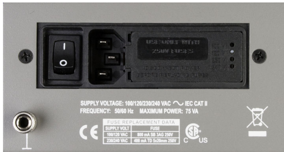
Figure 2. Detail, power entry module on APx515 instrument rear panel. The mains power switch is to the left.
