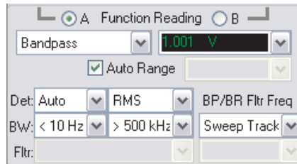
Figure 113. Analog Analyzer Function meter, Bandpass function.
