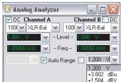
Figure 105. Analog Analyzer input ranging.
