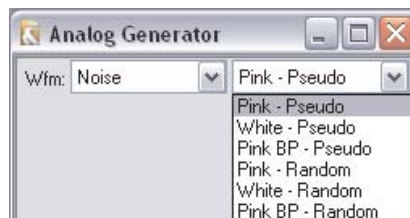
Figure 52. Analog Generator Wfm: Noise Waveform Selections (S2-BUR hardware-generated signals)
