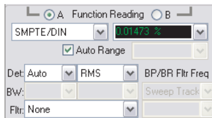
Figure 117. Analog Analyzer Function meter, SMPTE/DIN function.
