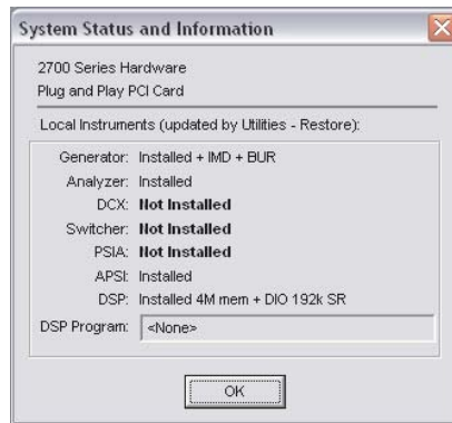
Figure 176. Hardware Status panel confirming installation of APSI hardware.
