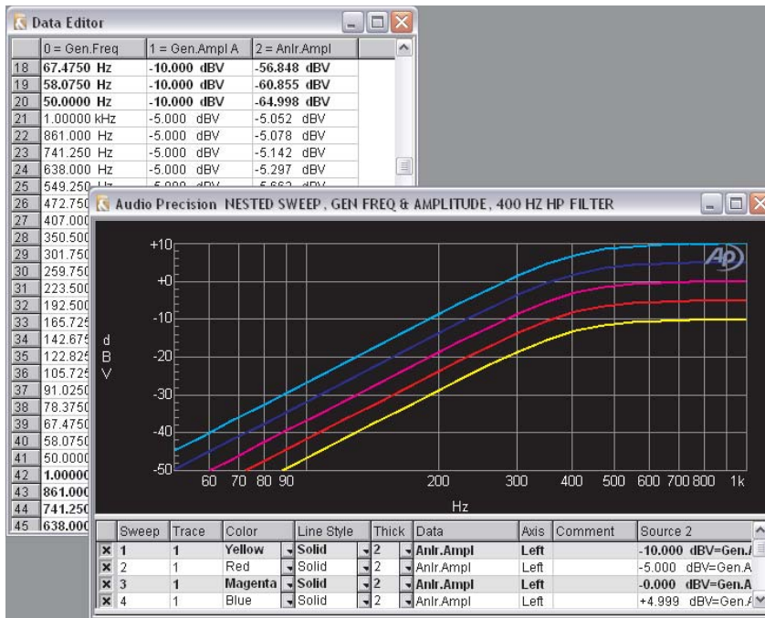
Figure 351. Graph Legend and Data Editor, showing the linked relationship of the typefaces used in the two displays, for a nested sweep.
