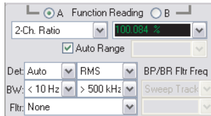
Figure 122. Analog Analyzer Function meter, 2-Ch. Ratio function.
