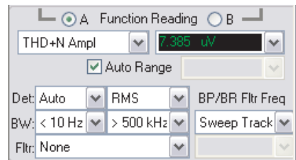
Figure 115. Analog Analyzer Function meter, THD+N Ampl function.
