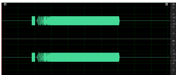
Time aligned waveforms. Channels 1 and 2 begin within a few ms of each other.
