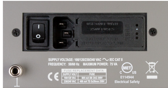
Figure 2. Detail, power entry module on APx515 instrument rear panel. The mains power switch is to the left.
