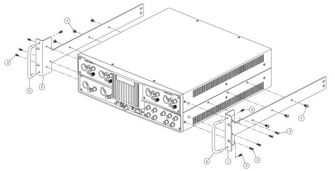
Figure 2. Fixed rackmounting installation
