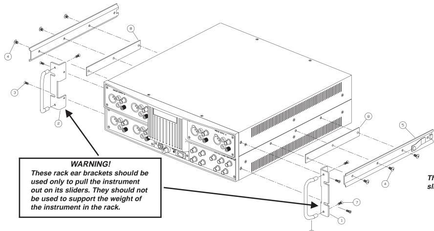
Figure 1. Slide-out racknounting installation
