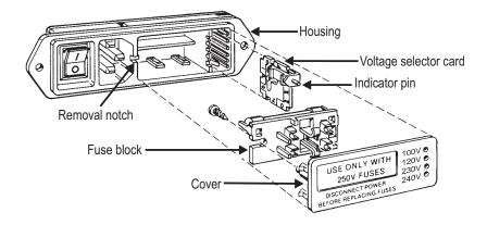
Figure D-2. Exploded Diagram of Power Entry Module
