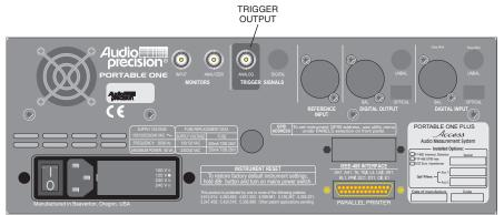
Figure 3-4. Rear Panel with Trigger Output Marked
