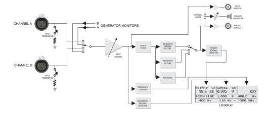
Figure 4-21. Block Diagram of SINAD Measurement
