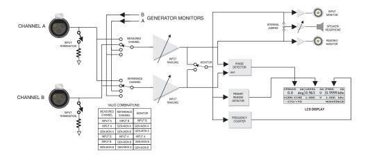
Figure 4-23. Block Diagram of Phase Measurement
