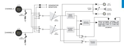
Figure 4-28. Block Diagram of RATIO Measurement
