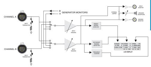
Figure 4-17. Block Diagram of LEVEL Measurement
