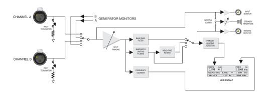
Figure 4-13. Block Diagram of Amplitude Measurement
