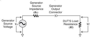
Figure 4-10. Source and Load Impedances
