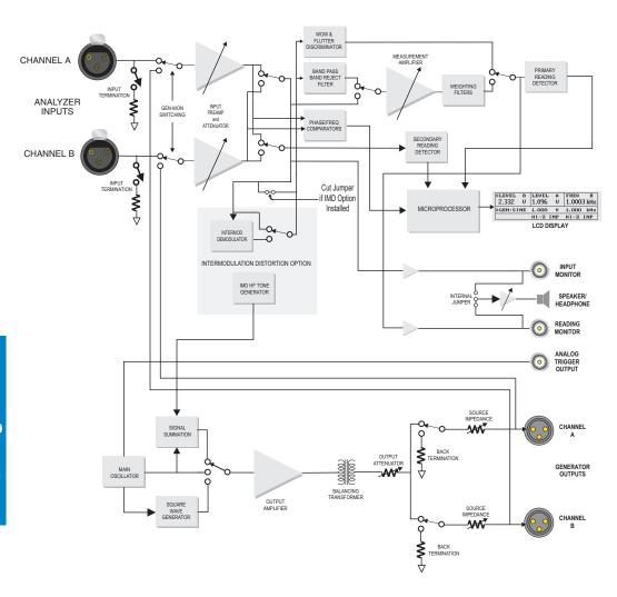
Figure 6-1. Instrument Block Diagram
