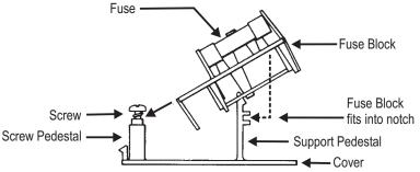
Figure D-4. Insertion/Removal of Fuse Block
