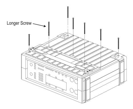
Figure B-1. Screws Removed for Case Disassembly
