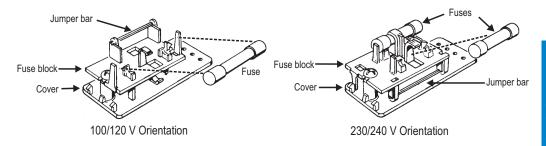
Figure D-5. Fuse Block Orientations
