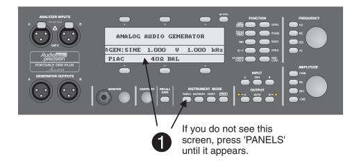
Figure 3-3. Selecting output impedance
