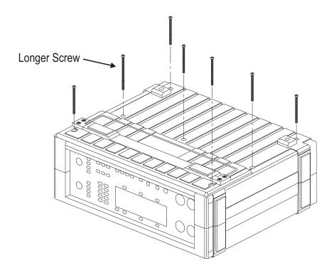
Figure C-1. Screws Removed for Case Disassembly
