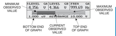
Figure 4-37. Bargraph Screen in Level Function
