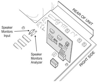
Figure C-2. Monitor Selection Resistor Positions
