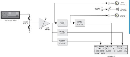
Figure 4-34. Block Diagram of AC Mains Measurement
