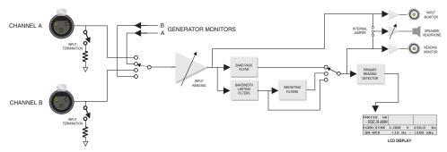
Figure 4-15. Block Diagram of NOISE Measurement
