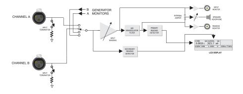
Figure 4-25. Block Diagram of IMD Measurement
