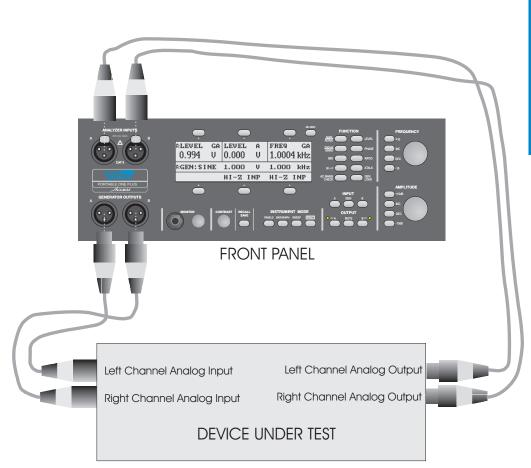
Figure 2-7. Typical Connections to Device-Under-Test
