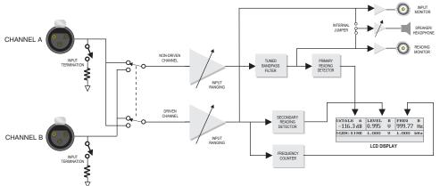
Figure 4-32. Block Diagram of Crosstalk Measurement
