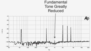
The fundamental tone has been reduced to a level where it will be insignificant. The filtered signal is then measured with another voltmeter, and the reading is presented as a ratio of the two voltmeter readings.
