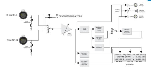
Figure 4-19. Block Diagram of THD+N Measurement
