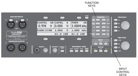
Figure 4-11. Analyzer Control Keys
