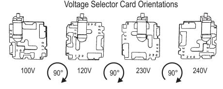
Figure D-3. Proper Orientations for Selector Card
