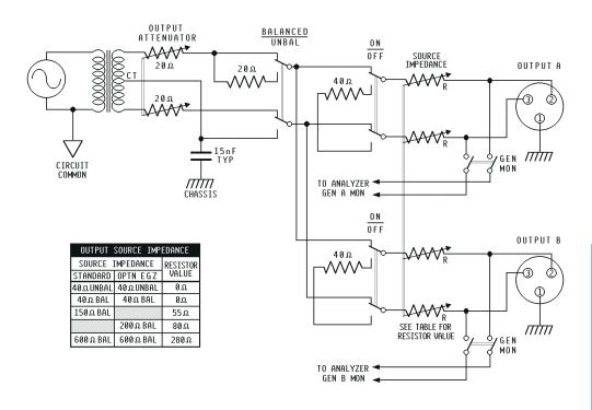
Figure 6-2. Simplified Analog Generator Output Circuit
