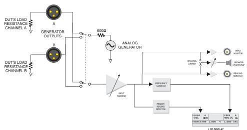
Figure 4-36. Block Diagram of Generator Loading Measurement
