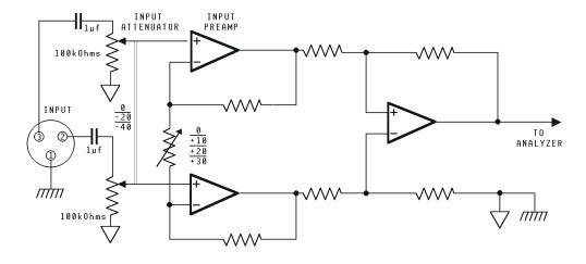
Figure 6-3. Simplified Analog Analyzer Input Circuit
