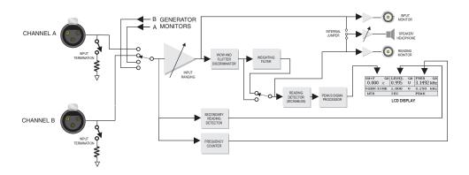
Figure 4-30. Block Diagram of Wow and Flutter Measurement
