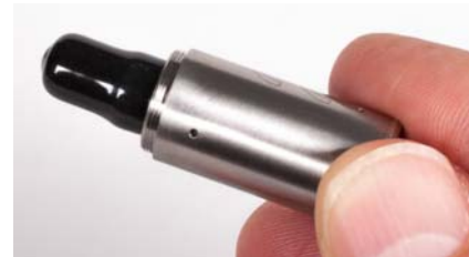
Figure 19. Protective rubber boot on preamplifier threads
