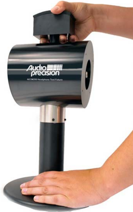
Figure 21. Separating the head from the neck.
