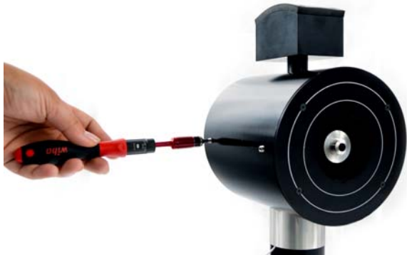
Figure 31. Tightening the ear simulator clamp set screws.
