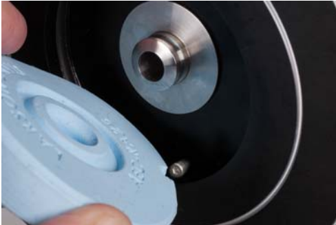
Figure 9. Aligning the pinna.
