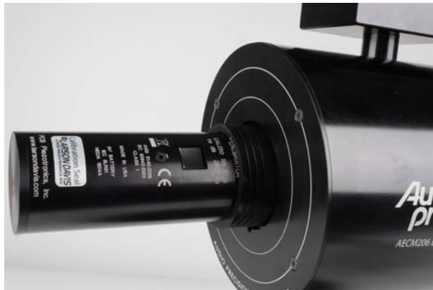
Figure 11. CAL250 attached to the AECM206
