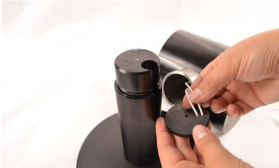
Figure 26. Inserting the cables into the gasket.
