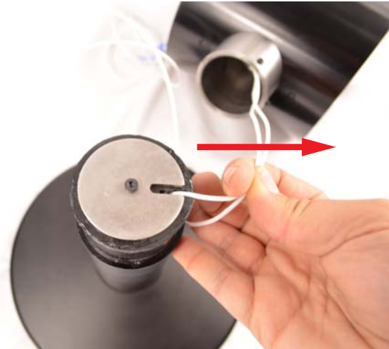
Figure 23. Slip the cables through the slot in the gasket and then pull the cables up through the opening in the neck.
