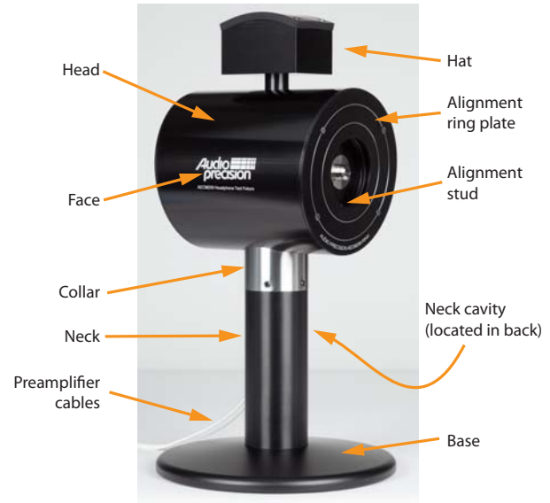
Figure 2. Headphone Test Fixture key components
