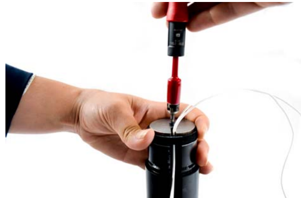
Figure 27. Tightening the neck washer and gasket.
