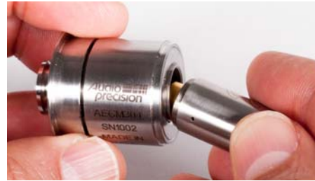
Figure 18. Separating the preamplifier and ear simulator
