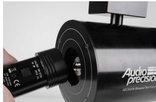
Figure 13. Removing the calibrator.
