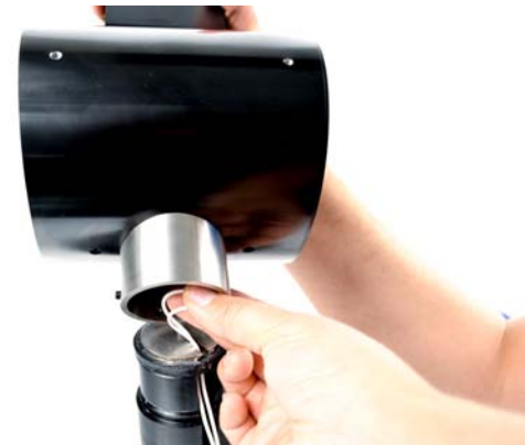
Figure 30. Feeding cable slack into the head cavity.
