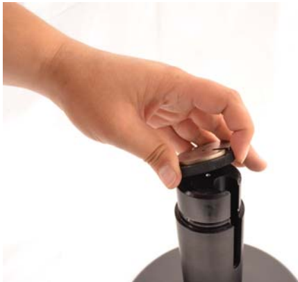
Figure 24. Removing the neck washer and gasket.
