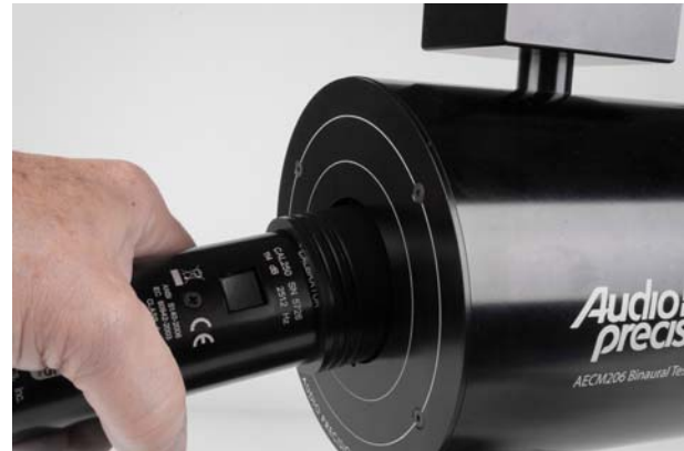
Figure 12. Pressing down to release gasket seal.
