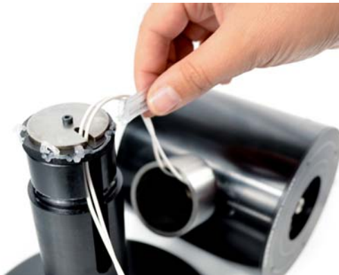
Figure 28. Applying silicon grease to the neck gasket (1).
