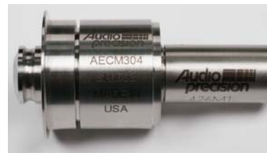
Figure 6. An AECM304, shown here fitted with an ear canal extension to the left in the photograph, and mated to an 426M15 preamplifier, shown to the right. Two such assemblies are mounted within the AECM206 head.
