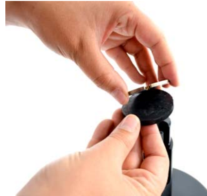
Figure 25. Separating the washer from the gasket.
