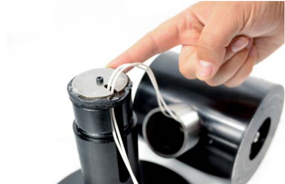
Figure 29. Applying silicon grease to the neck gasket (2).
