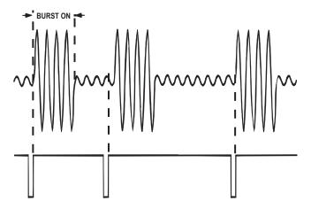
Figure 4-6 Burst Triggered Mode, Definitions
