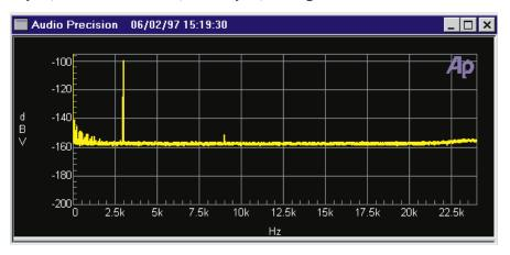
Figure 15-7 Same Low Level Signal, 128x Power (Spectrum only) Averaging. Noise Variance is Reduced, No Change in Average Noise Level
