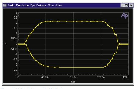
Figure 8-12 Eye Pattern (48 kHz Rate)
