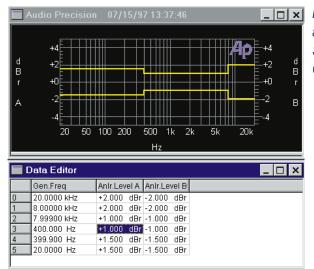
Figure 22-4 Data Editor and Graph Viewed Simultaneously While Creating Limits File
