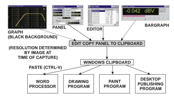
Figure 21-15 Schematic Representation of Various Hardcopy Techniques
