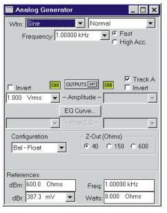
Figure 4-2 Analog Generator Panel, Large Version
