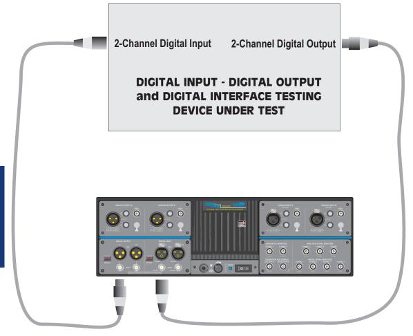
A System Two Cascade Dual Domain (SYS-2522) series instrument is required for these tests. A standard installation places System Two Cascade digital interface tests in the
