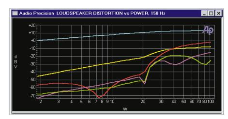
Figure 12-3 Fundamental (top curve), 2nd harmonic, 3rd harmonic, 4th harmonic, and 5th harmonic amplitudes of a loudspeaker as a function of power.
