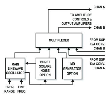
Figure 4-15 Oscillator Section, System Two Analog Generator
