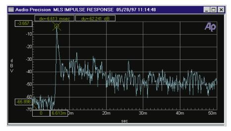
Figure 17-3 Loudspeaker Impulse Response, Showing 6.6 Millisecond Delay to Impulse Peak. This Waveform Furnished as C:\APWIN\S1\PROCEDUR\DEMO\THREEWAY.AAM
