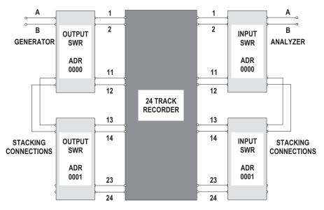
Figure 25-2 Switcher Connection and Address Setting Diagram, Multi-track Recorder
