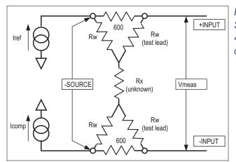
Figure 26-6 Simplified diagram of 4-wire ohmmeter operation
