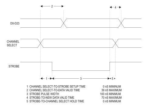
Figure 9-3 Parallel Output Port, Timing Relationships
