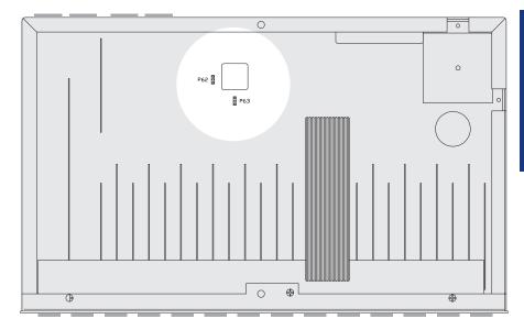
Figure 25-16 P62 and P63 Jumper Locations Inside SWR-2122 Switchers
