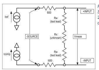
Figure 26-5 Simplified diagram of 2-wire ohmmeter operation
