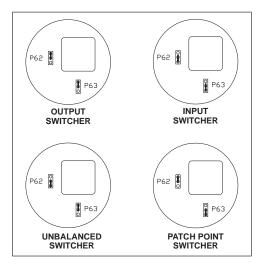
Figure 25-17 P62 and P63 Jumper Placement for Output, Input, Patch Point, and Unbalanced Switchers
