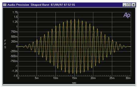
Figure 4-10 Shaped Burst Example
