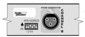
Figure 25-18 Rear panel DIP switch (typical)
