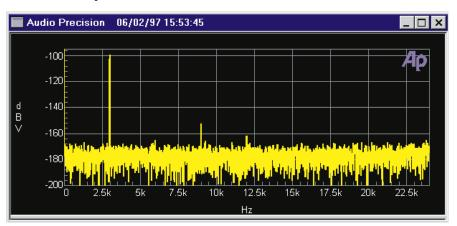
Figure 15-8 Same Low Level Signal, 128x Synchronous (Time Domain) Averaging. Average Noise Level is Reduced, No Change in Noise Variance
