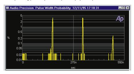
Figure 8-13 Interface Pulse Width (Interface Timing) Probability, 48 kHz Rate
