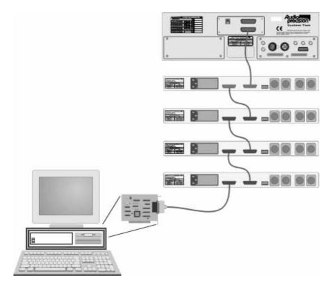
Figure 25-15 APIB connections block diagram (typical)
