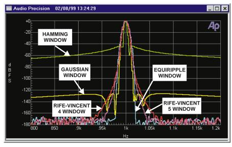
Figure 15-4 Additional Window Functions Available with System Two Cascade, FFT; Equiripple Shown in Both Figures for Comparison
