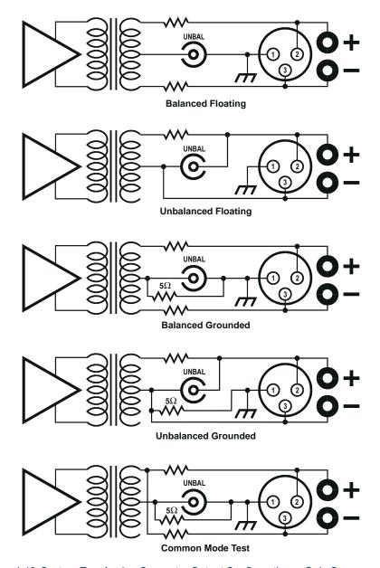
Figure 4-13 System Two Analog Generator Output Configurations. Only One Channel Shown; Both Channels Identical
