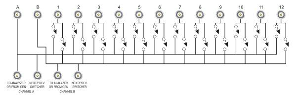
Figure 25-11 SWR-2122U Unbalanced Switcher simplified schematic
