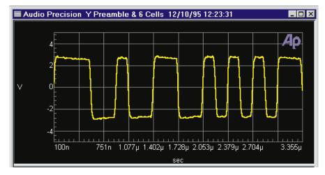
Figure 8-9 Interface Waveform. Y Preamble (3 UI-2 UI-1 UI-2 UI) Followed by Six Data Cells (0,0,1,1,1,0)
