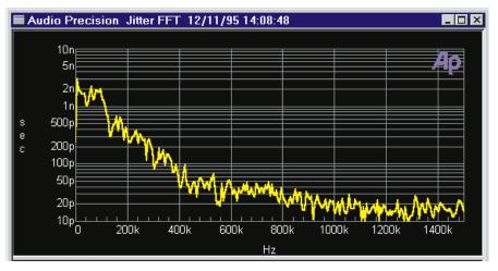
Figure 8-10 FFT Spectrum Analysis of Jitter Signal (100 kHz Lowpass Random Noise from System Two Jitter Generator)
