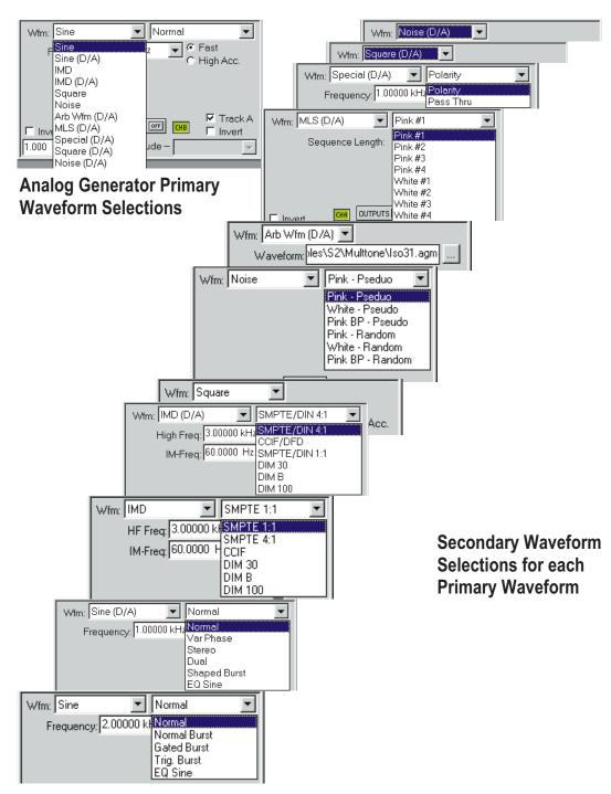
Figure 4-3 Analog Generator Waveform Selection
