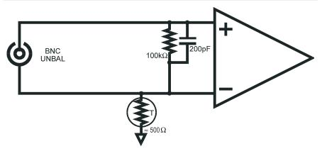
Figure 5-20 System Two Analyzer Equivalent Input Circuit, Unbalanced BNC
