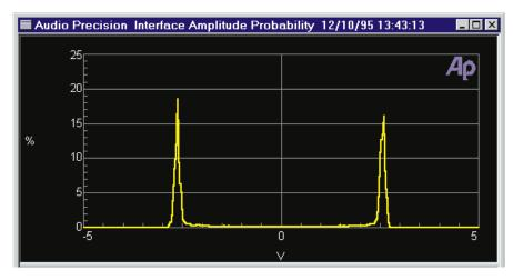
Figure 8-15 Probability vs Amplitude (5 V p-p Interface Signal)
