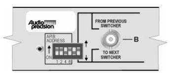
Figure 25-19 Unbalanced switcher address/mode switch
