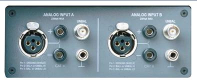
Figure 1-4 Analog Analyzer (Upper Right) Input Connector Panel
