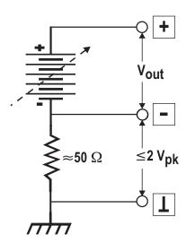
Figure 26-7 Equivalent Circuit, DC Outputs 1 or 2
