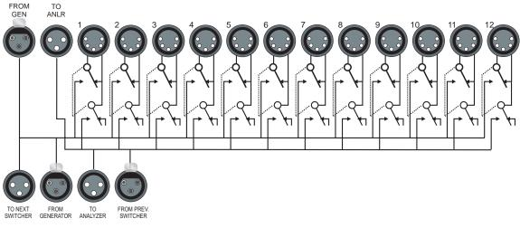
Figure 25-14 SWR-2122P Patch-Point Switcher simplified schematic
