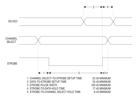
Figure 9-2 Parallel Input Port, Timing Relationships
