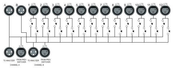
Figure 25-5 Input Switcher simplified schematic
