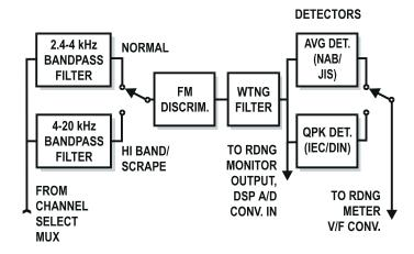
Figure 5-8 Wow and Flutter Analyzer Option, Simplified Diagram
