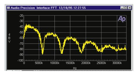
Figure 8-8 FFT Spectrum Analysis of Serial Interface Signal (48 kHz Rate)
