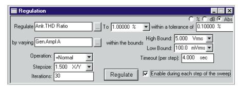
Figure 3-4 Regulation Panel, Typical Setup for Power Bandwidth Sweep
