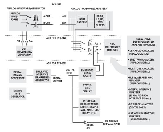
Figure 1-1 Conceptual Block Diagram, System Two
