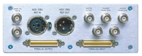
Figure 18-2 System Two Cascade DSP Rear Panel
