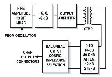
Figure 4-16 System Two Analog Generator Output Stage (Channels A and B Indentical)
