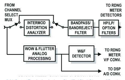
Figure 5-21 System Two Analog Analzyer, Simplified Block Diagram of Function
