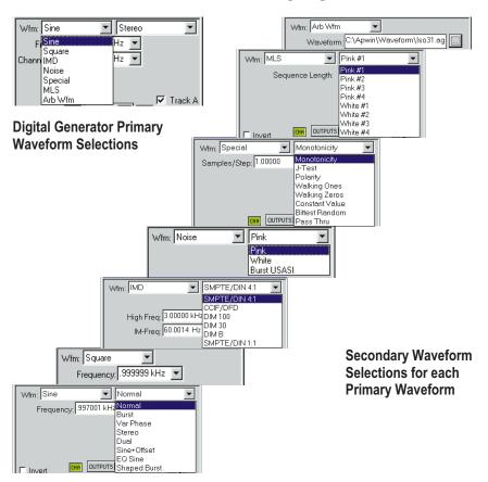
Figure 10-3 Digital Generator Waveform Selections
