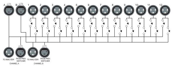
Figure 25-8 Output Switcher simplified schematic
