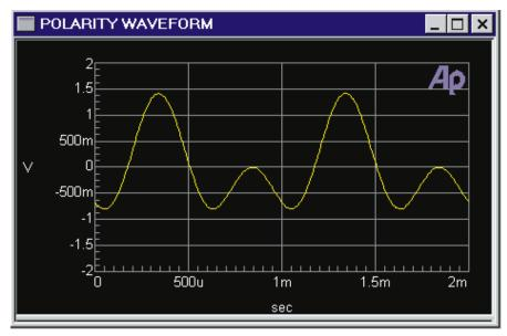
Figure 4-11 Polarity Waveform, No Inversion
