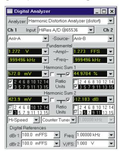
Figure 12-1 Harmonic Distortion Analyzer Panel, Large Form
