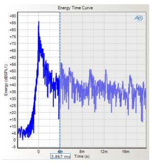
individual harmonic. Chirp has a big advantage here over the old MLS (maximum length sequence) method, in that distortion can be distinguished from the fundamental. This makes accurate frequency response measurement, as well as detailed distortion analysis, possible.
