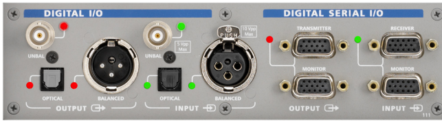
Figure 1 APx Digital I/O and Digital Serial I/O front panel
