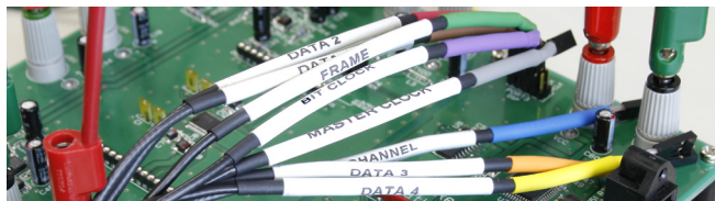
Figure 2 APx DSIO Clock and data lines.
