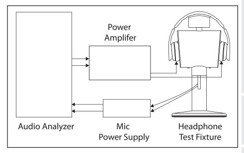
Simplified diagram of a headphone testing application, with an audio power amplifier, an audio analyzer and a microphone power supply.
