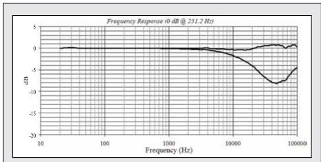
Typical free-field response of the microphone with the grid cap at 0 degree incidence. The top curve is the corrected free-field curve, and the bottom curve is the pressure response generated by the electronic actuator.
