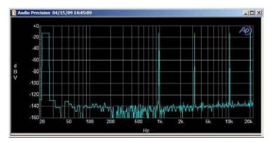
An FFT of the High Speed Tester multitone with tones at approximately 20 Hz, 1 kHz, 3 kHz, 10 kHz and 20 kHz.
