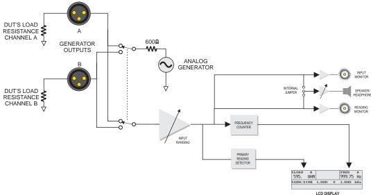
Figure 4-38 Block Diagram of Generator Loading Measurement
