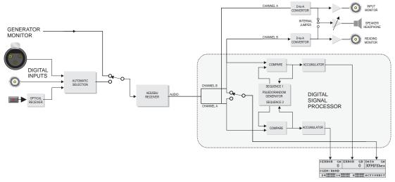
Figure 4-43 Block Diagram of Data Check Measurement
