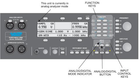
Figure 4-13 Analyzer Control Keys
