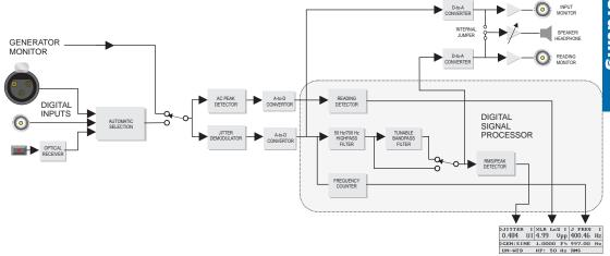
Figure 4-40 Block Diagram of Jitter Measurement
