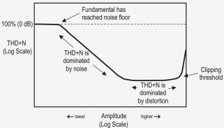
Note that for some low-distortion devices, the flat area before clipping may shrink or not exist at all. The THD+N measurement may be noise-dominated at all amplitudes below the clipping threshold.
