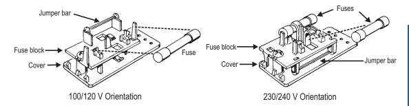
Figure 10-5 Fuse Block Orientations
