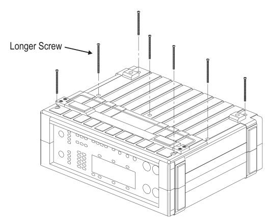
Figure 9-1 Screws Removed for Case Disassembly
