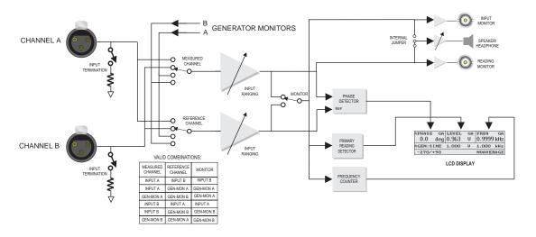
Figure 4-25 Block Diagram of Analog Phase Measurement
