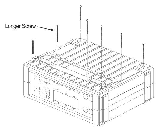
Figure 8-1 Screws Removed for Case Disassembly
