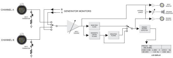
Figure 4-17 Block Diagram of Analog NOISE Measurement
