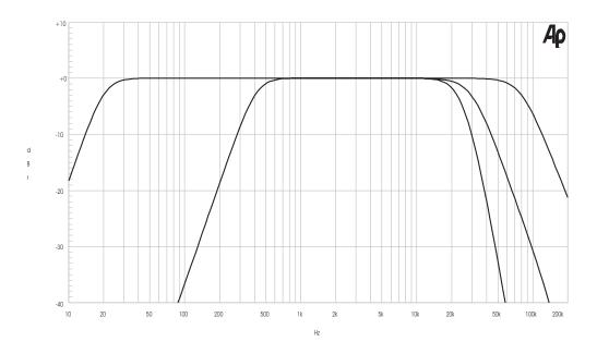
Shapes of Bandwidth Limiting Filters - 22 Hz Highpass, 400 Hz Highpass, 22 kHz Lowpass, 30 kHz Lowpass, 80 kHz Lowpass.
