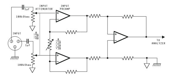
Figure 6-4 Simplified Analog Analyzer Input Circuit
