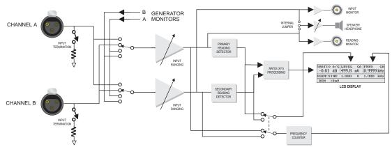
Figure 4-30 Block Diagram of Analog RATIO Measurement
