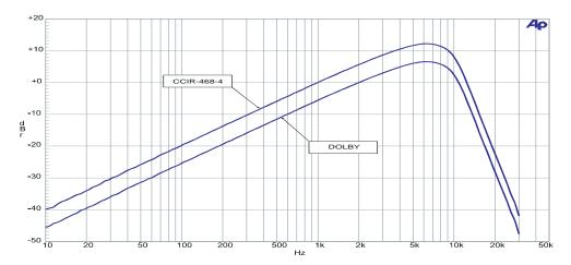
Shape of CCIR Filter - CCIR-468-4 has the 0 dB point at 1 kHz, while the Dolby curve has the 0 dB point at 2 kHz.
