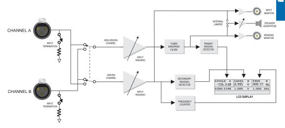
Figure 4-34 Block Diagram of Analog Crosstalk Measurement
