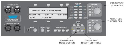
Figure 4-9 Generator Controls
