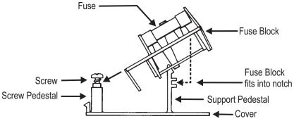
Figure 10-4 Insertion/Removal of Fuse Block
