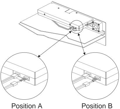
Figure 9-2 Cable Positions for Monitor Selection
