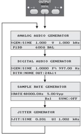
Figure 4-10 Generator Control Modes (Generator Only Panel)
