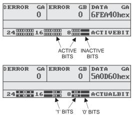
Figure 4-45 Appearance of Bits in Data Check Mode
