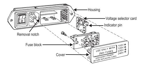
Figure 10-2 Exploded Diagram of Power Entry Module
