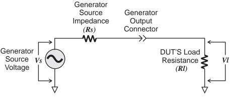
Figure 4-11 Source and Load Impedances
