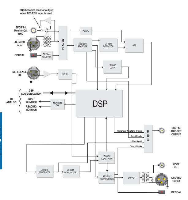
Figure 6-2 Digital Block Diagram
