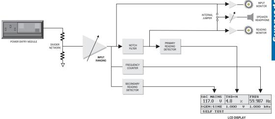
Figure 4-36 Block Diagram of AC Mains Measurement
