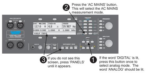
Figure 12-1 Steps to the Main Panel in AC Mains Function
