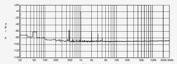
After the bandpass filter eliminates the 1 kHz fundamental tone, we are left with the following:
