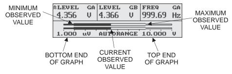
Figure 4-50 Bargraph Screen in Level Function
