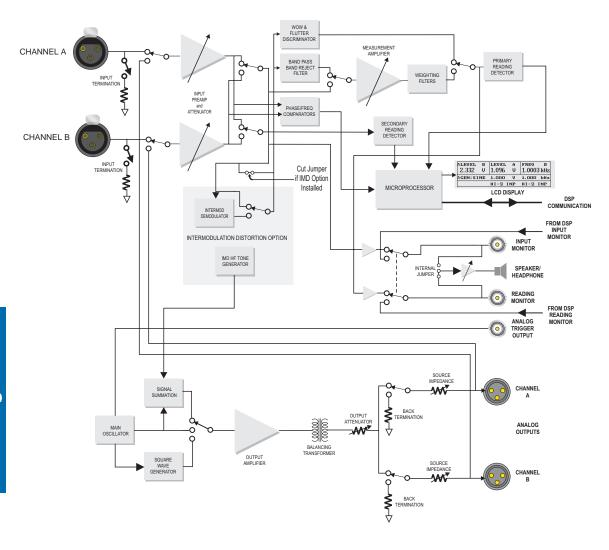
Figure 6-1 Analog Block Diagram
