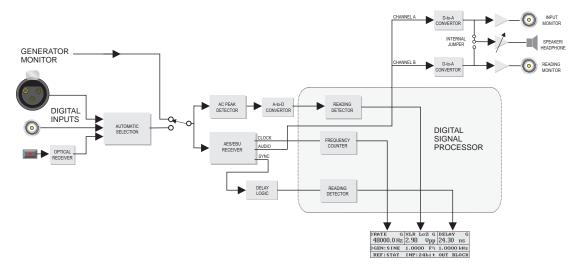
Figure 4-42 Block Diagram of Digital I/O Measurement
