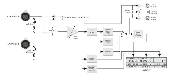
Figure 4-23 Block Diagram of Analog SINAD Measurement
