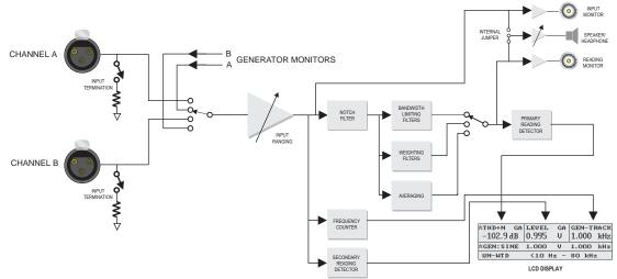
Figure 4-21 Block Diagram of Analog THD+N Measurement
