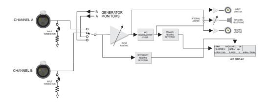
Figure 4-27 Block Diagram of Analog IMD Measurement
