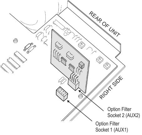
Figure 8-2 Location and Orientation of Option Filters
