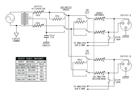
Figure 6-3 Simplified Analog Generator Output Circuit
