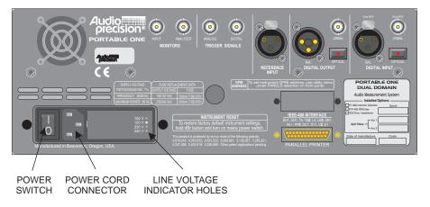
Figure 10-1 Rear Panel Showing AC Mains-Related Components
