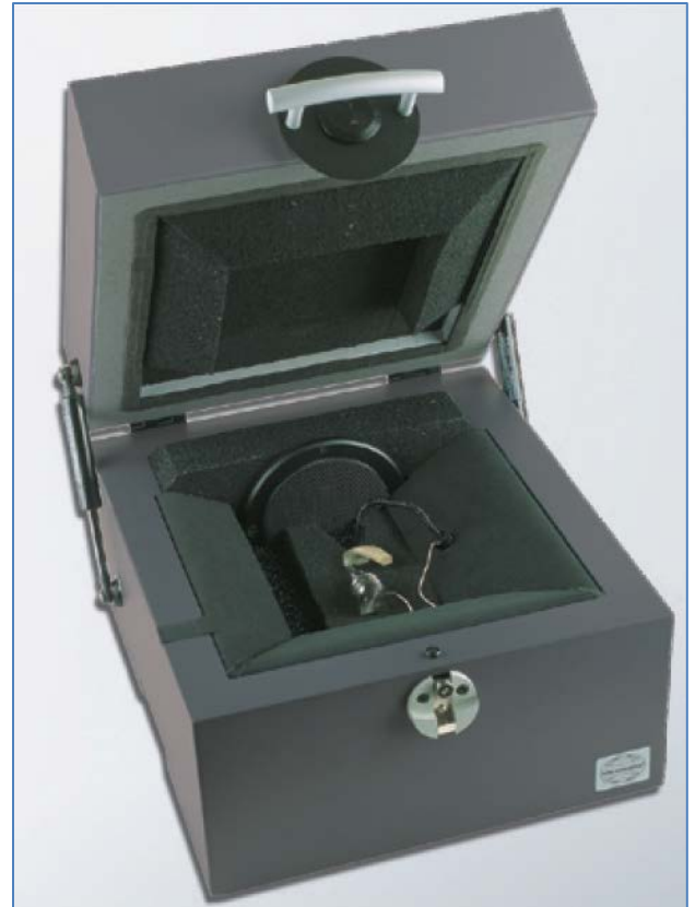
Figure 3. An Interacoustics TBS25 Test Chamber.
