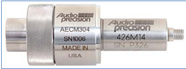
Figure 2. An occluded ear simulator (per IEC 60318-4) with attached microphone preamplifier.
