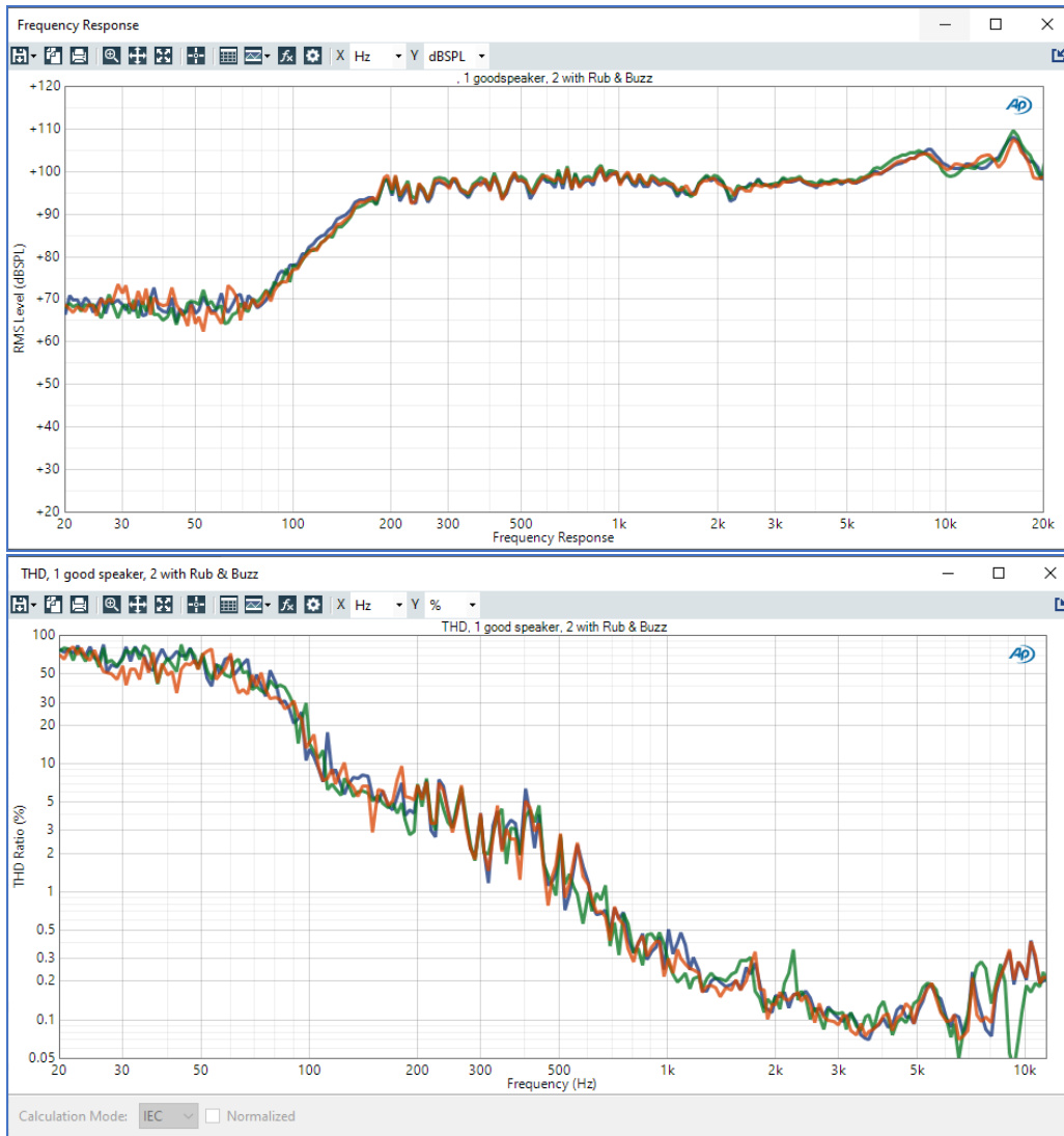
Figure 2. Graphs of frequency response (upper) and THD response (lower) of three samples of a small driver – one with no audible defects and two with audible rub and buzz distortion.
