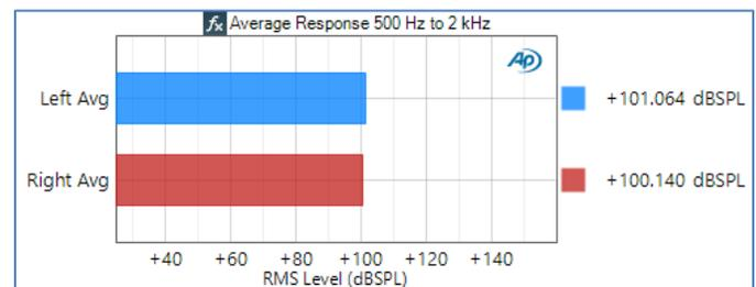
Figure 17. Headphone response averaged from 500 Hz to 2 kHz.
