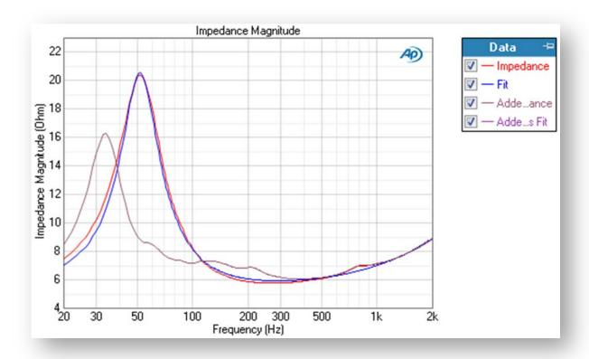
This is the impedance curve of a driver in the Impedance/Thiele-Small measurement. The larger curve is the free-air measurement; the smaller curve shows the lowered resonance frequency when the driver is measured with added mass.
